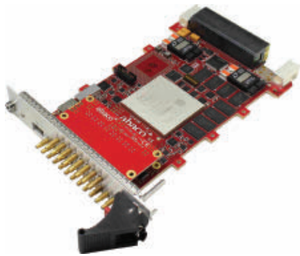
The Abaco 3U VPX VP430 direct RF processing system is one of the densest analog FPGA DSP boards available, with eight A/D and D/A synchronized channels.
